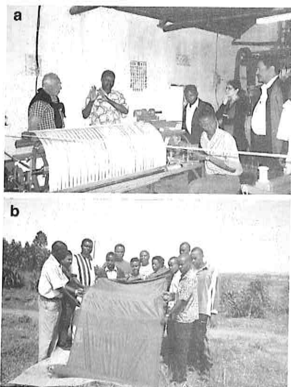
Figure 5. Post-cocoon operations at Bushenyi Silk Marketplace, Uganda: (a) a trained weaver develops silk warp for weaving; (b) BSFA farmers unfolding silk cloth from the beam
