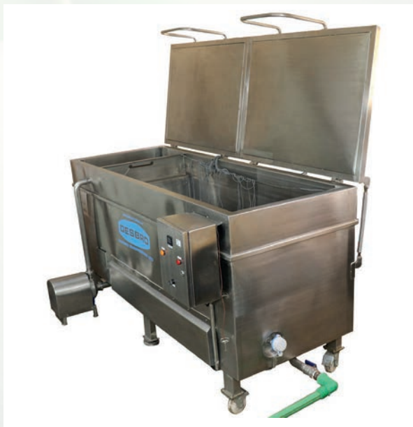
Plate 16: A miniature Hot water treatment tank with temperature controls/sensors, a water pump for water circulation, and cladded walls to guard against heat loss during treatment
